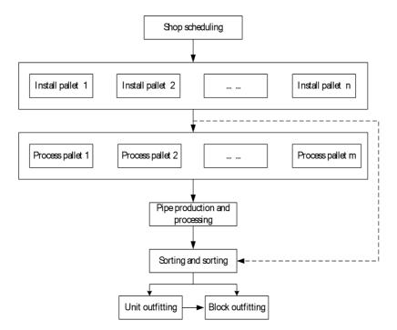
Fig. 1. Management mode of double tray in pipe workshop
