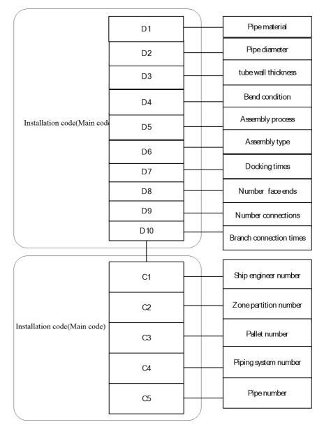
Fig. 5. Pipe coding structure based on double pallet management
