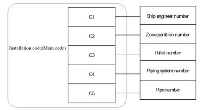
Fig. 3. Tube-oriented structure for the installation
